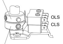
CLS CAM (CLOSE LIMIT SWITCH CAM)
